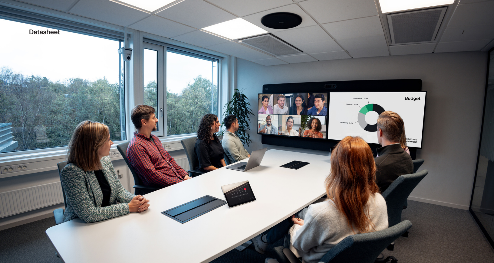
Figure 4. A Room Kit EQX with 65" dual screens in combined deployment with a Ceiling Microphone Pro for directional speech capture.
